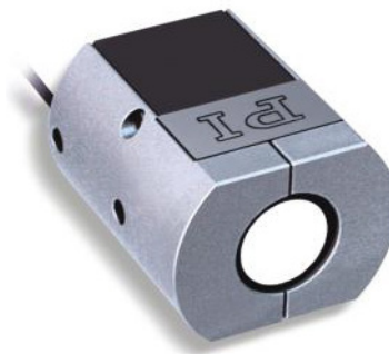
Fig. 3 Compact piezo tip/tilt mirror with two orthogonal axes and 100 mrad optical deflection angle with 0.0005 mrad resolution; length 38 mm (Image: PI)
